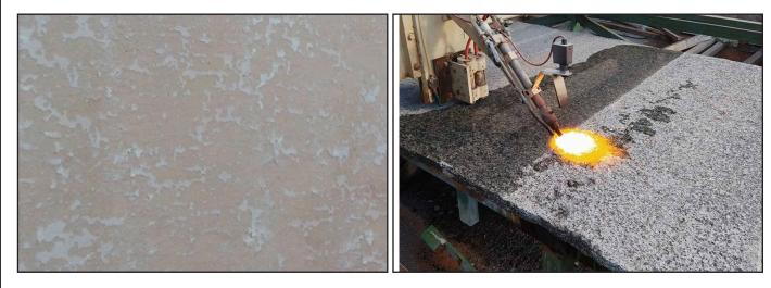
**Flamed:** Applying blowtorch-strength heat to the surface of Marble & Granite, this actually pops some of the crystals and creates a deeply textured surface which produces flamed Stone.
